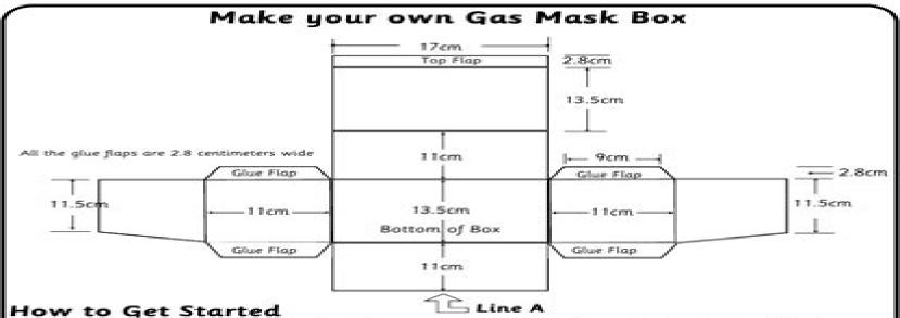
Take a large sheet of stiff brown card and draw out the net shown above to the right size. Mark the middle of the bottom edge of the card and place the centre of Line A there. Continue to draw the rest of the net and carefully cut it out. Score along the remaining lines as they are folds. Fold up your box and glue the Glue Flaps, they go inside the long sides of the box. The Top Lip tucks into the box and holds the top shut. Cut out the instructions below and stick them inside the lid.
