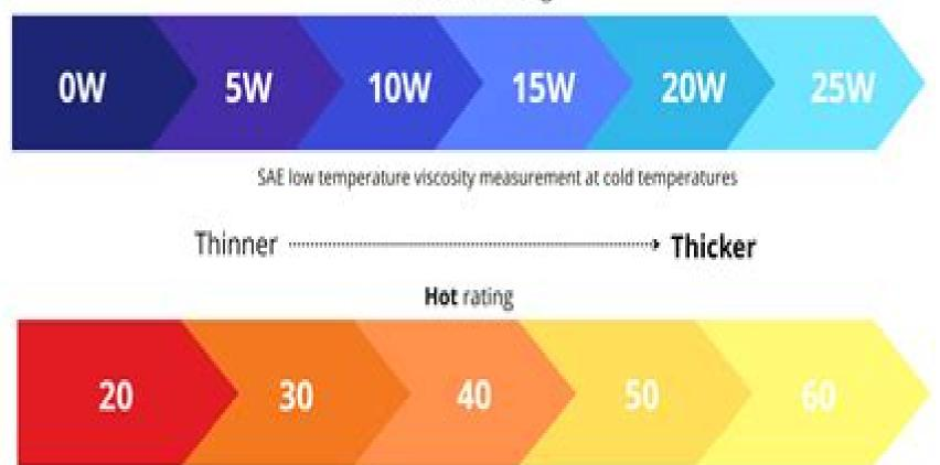
SAE high temperature viscosity measured at 100°C (Standard Operating Temp)
