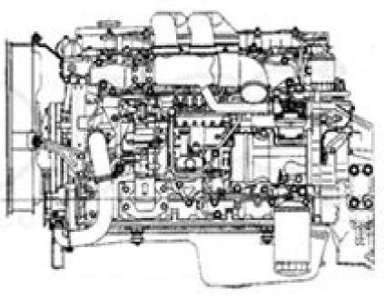
Diesel L6 / Direct Injection / 8,226 cm3 / 2 Value / OHC
