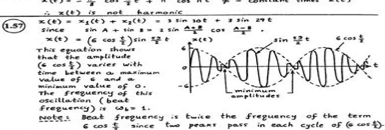
The resultant motion of two harmonic motions having identical amplitudes (X) but slightly different frequencies (
