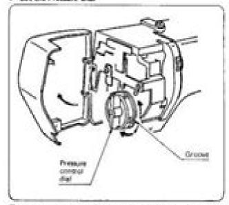
The pressure control dial is located inside the face cover plate.
