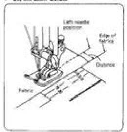
The seam guides on the needle plate are engraved to help you measure seam width.
