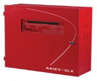
The ARIES-SLX annunciates alarm, trouble, and supervisory events via an 80-character, backlit LCD display with integral status LEDs. Event acknowledgment, alarm silence, and system reset are accomplished with dedicated control keys. Basic user and maintenance operations such as viewing history or isolation commands to initiating points and system outputs are performed via the control keys and associated digit keys. A security password prevents unauthorized access to the system.
