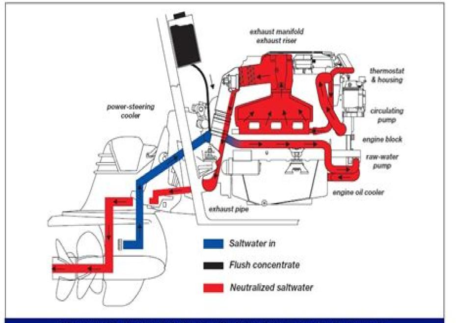
The new QL Neutra-Salt Engine Flushing System is now available for installation on all gasoline inboards and sterndrives.
