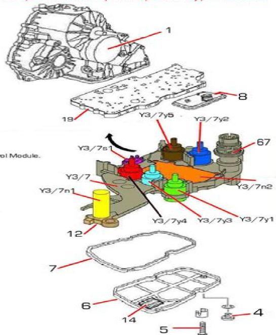
19 Shift Valve Housing. 67 Connector. Y3/7 Electric FTC Control Module. Y3/7n1 Trans output shaft RPM sensor. Y3/7n2 Front Wheel Drive. Transl [FTC] control Module. Y3/7s1 Starter Lockout contact. Y3/7y1 Shift 1/4 pulse-width-modulated solenoid Valve. Y3/7y2 Shift 3 pulse-width-modulated solenoid Valve. Y3/7y3 Shift 2/5R pulse modulated solenoid Valve. Y3/7y4 Torque converter lockup clutch pulse-width-modulated solenoid Valve. Y3/7y5 Shift pressure pulse-width-modulated solenoid Valve.
