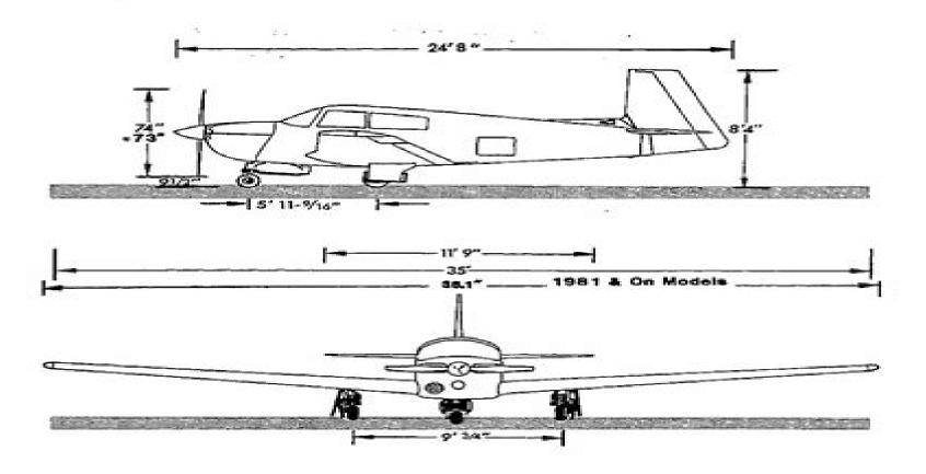
Figure 1-2. Principal Aircraft Dimensions M20 J. \* Optional Hartzell HC-C2YK-1BF propeller with F7666A-3Q blade.
