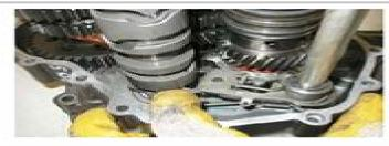
Unscrew and remove the threaded reference pin.
